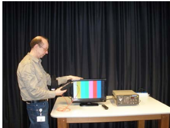
Current transformer clamped around arm of test person
