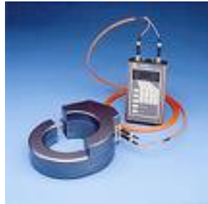
Figure 1 The Holaday clamp-on current probe HI-3702 and read-out system HI-4416
