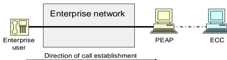
**Figure 2 — Example of an emergency call from an enterprise user to a PEAP**
