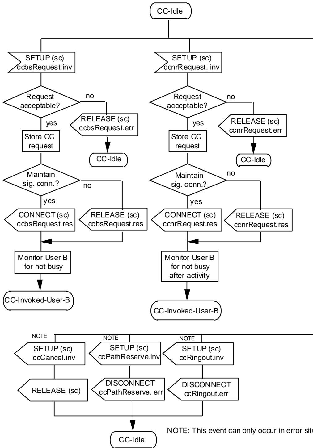
Figure D.11 - Terminating PINX behaviour
