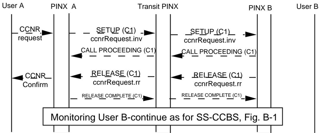
Figure C.3 - Example message flow for successful CCNR
