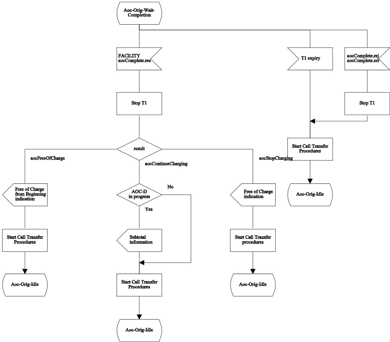
Figure C.4.2 - SDL Representation of SS-AOC at the Originating PINX - interaction with SS-CT (cont)
