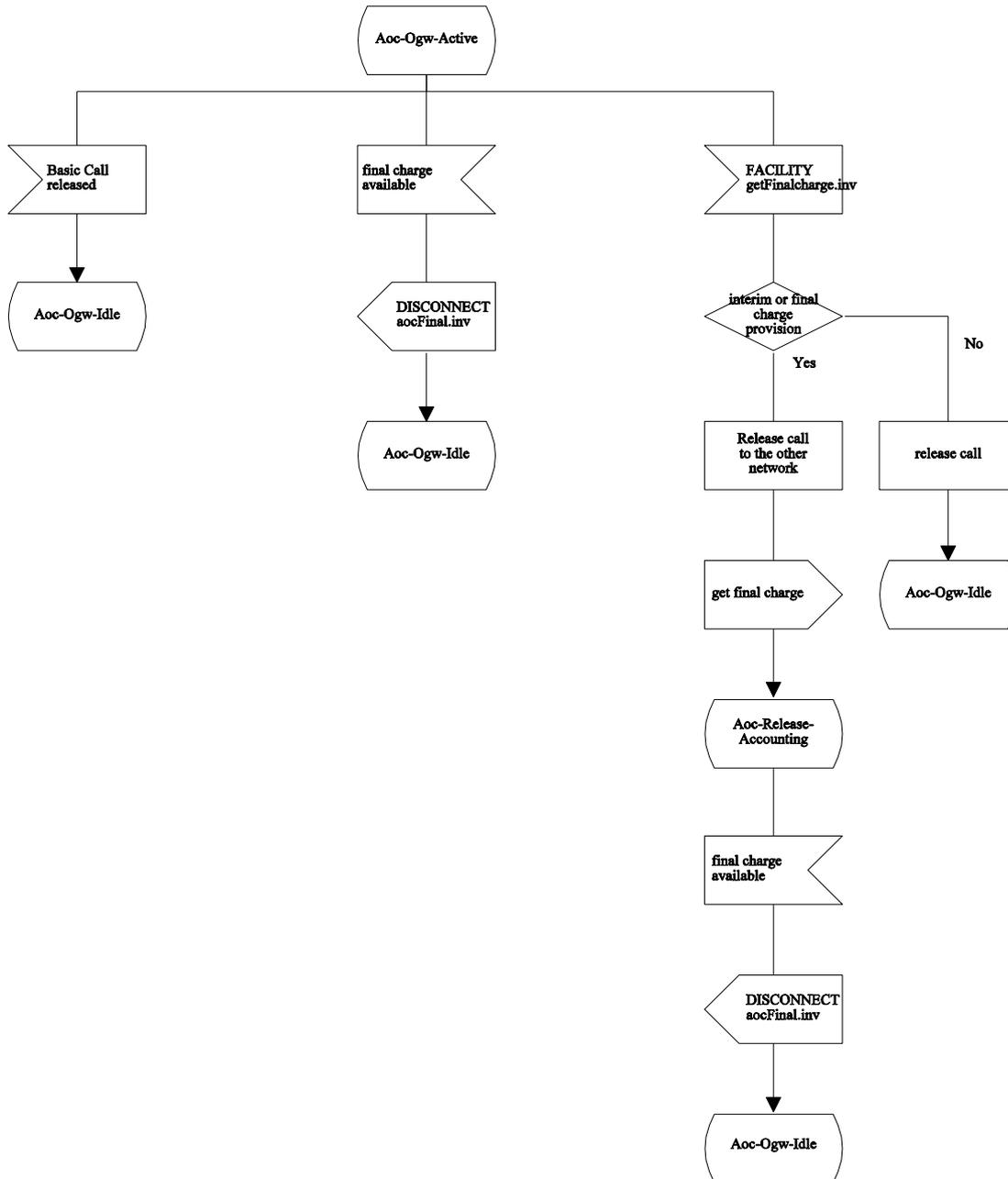
Figure C.2.2 - SDL Representation of SS-AOC at the Outgoing Gateway PINX (continued)
