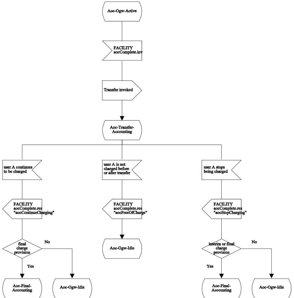
Figure C.2.4 - SDL Representation of SS-AOC at the Outgoing Gateway PINX (continued)
