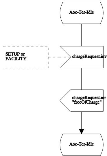
Figure C.3.1 - SDL Representation of SS-AOC at the Terminating PINX
