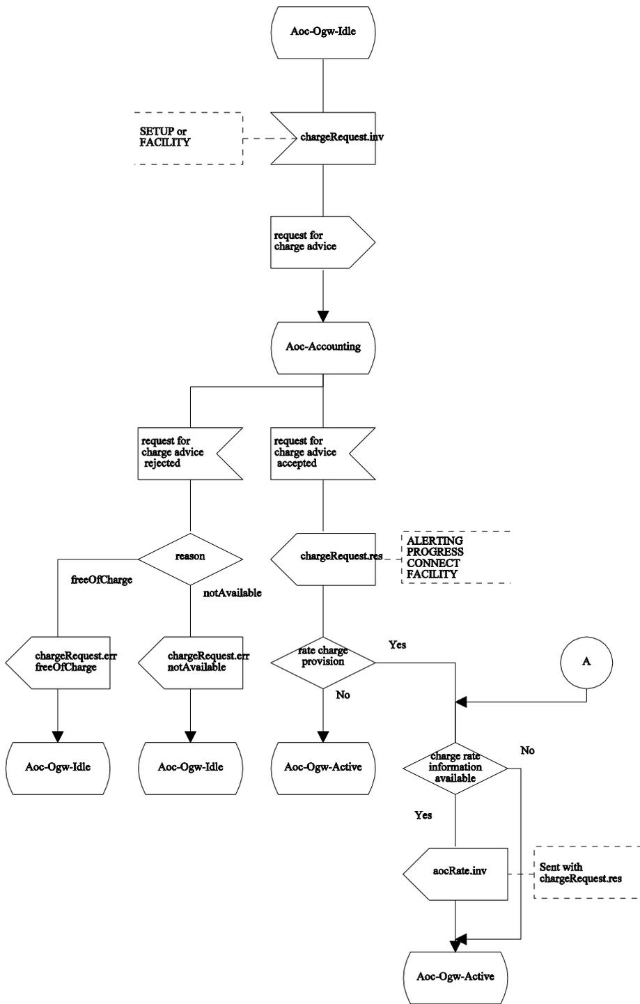
Figure C.2.1 - SDL Representation of SS-AOC at the Outgoing Gateway PINX
