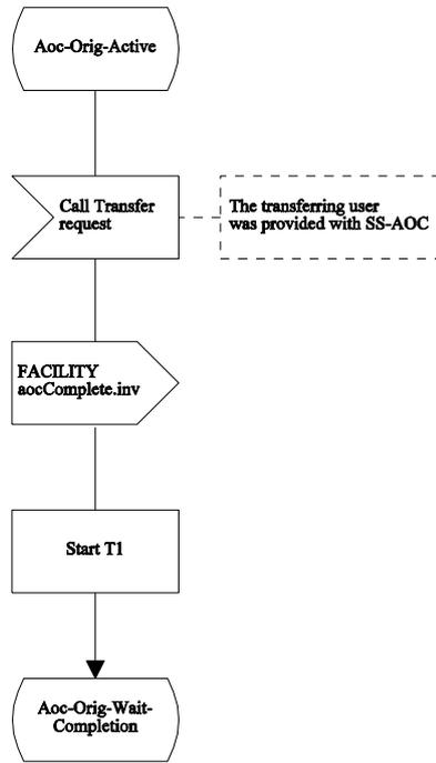
Figure C.4.1 - SDL Representation of SS-AOC at the Originating PINX - interaction with SS-CT
