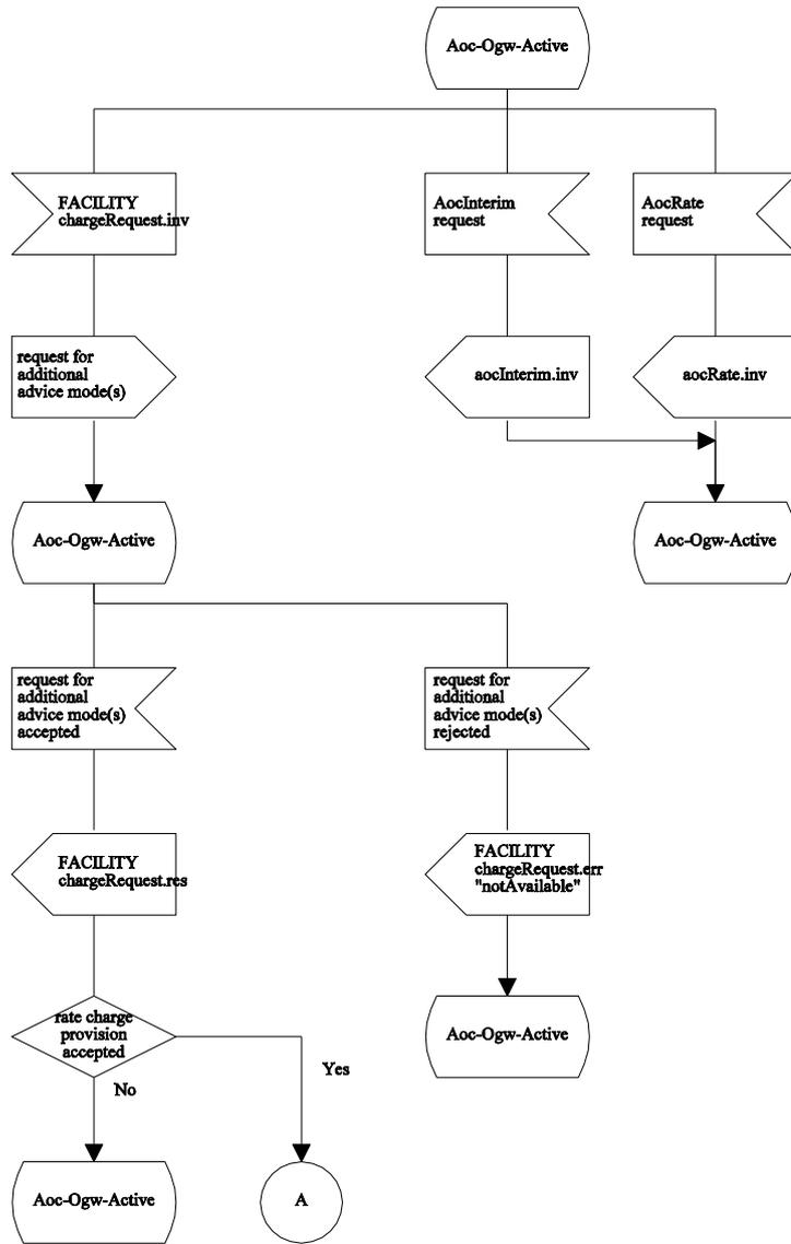
Figure C.2.3 - SDL Representation of SS-AOC at the Outgoing Gateway PINX (continued)
