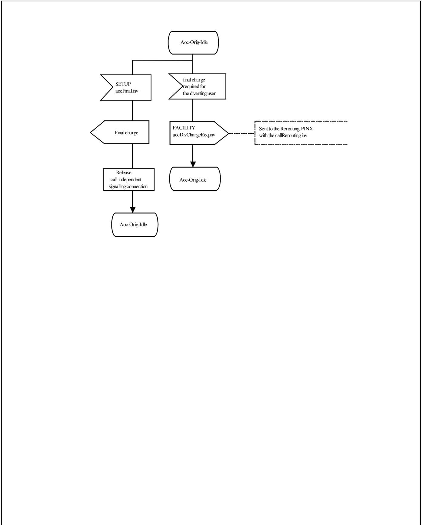
Figure C.5.1 - SDL Representation of SS-AOC at the Served User PINX - interaction with SS-DIV
