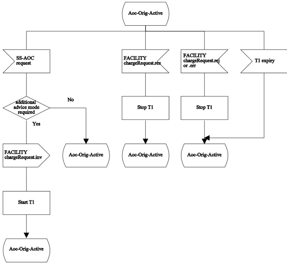
Figure C.1.4 - SDL Representation of SS-AOC at the Originating PINX (continued)
