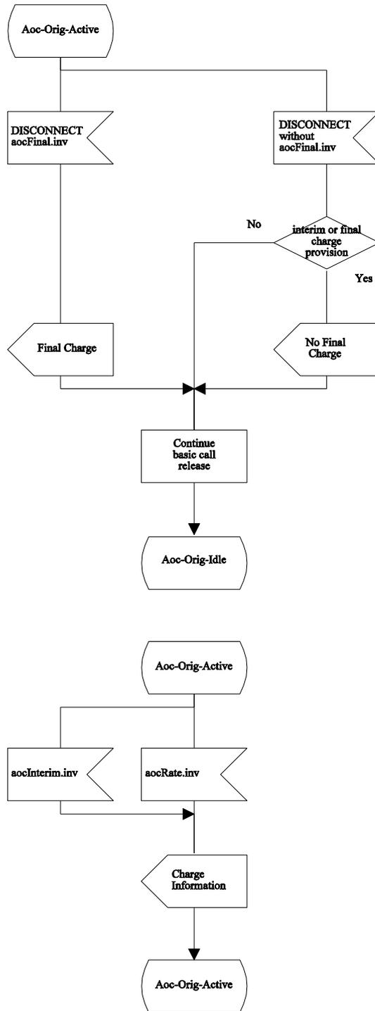
Figure C.1.3 - SDL Representation of SS-AOC at the Originating PINX (continued)
