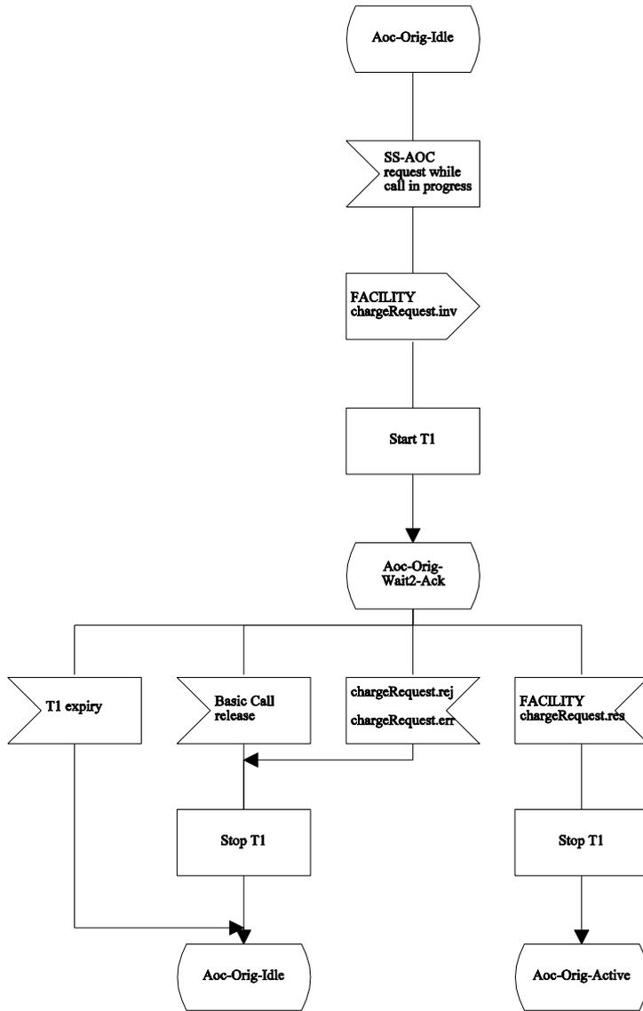
Figure C.1.2 - SDL Representation of SS-AOC at the Originating PINX (continued)
