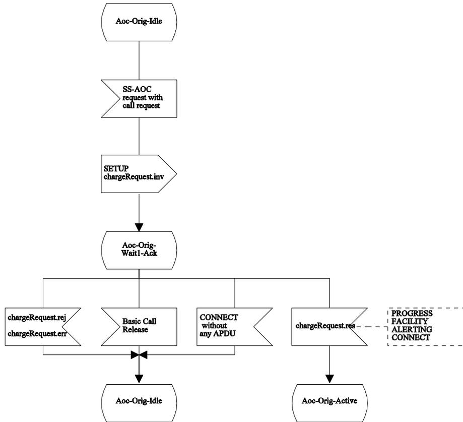
Figure C.1.1 - SDL Representation of SS-AOC at the Originating PINX
