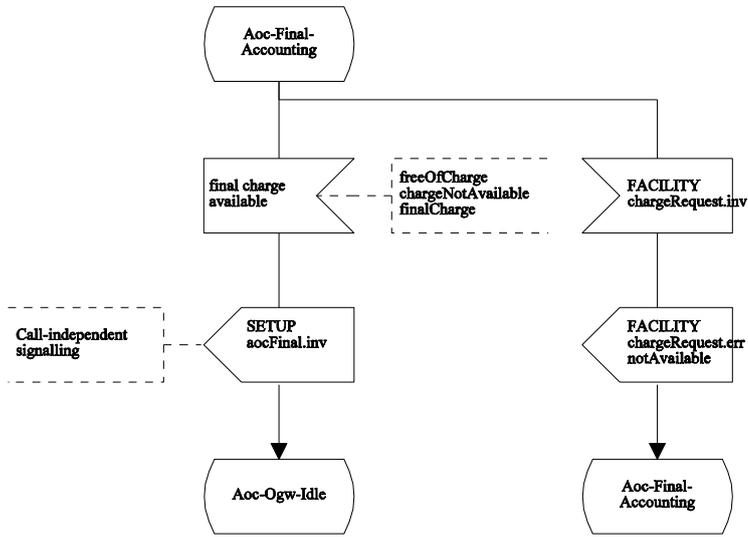
Figure C.2.5 - SDL Representation of SS-AOC at the Outgoing Gateway PINX (continued)
