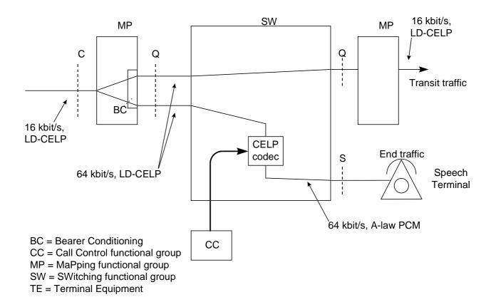
$Figure \ D.1 - Bearing \ conditioning \ and \ speech \ compression \ / \ decompression$
