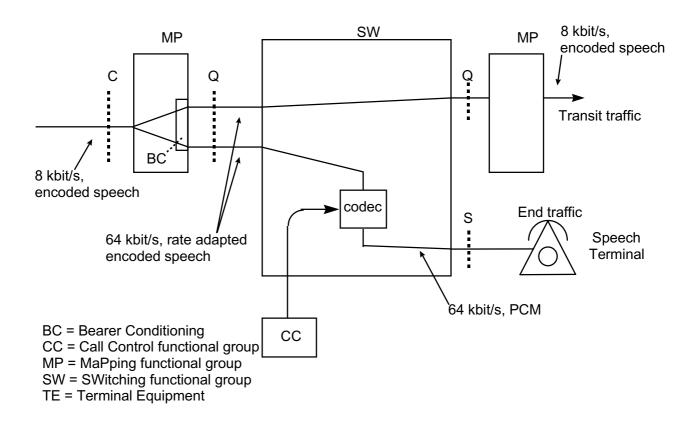
Figure D.1 - Example for the arrangement of bearer conditioning and speech compression / decompression
