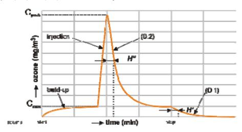
Figure D.1 — Application of equations (D.1) and (D.2)
