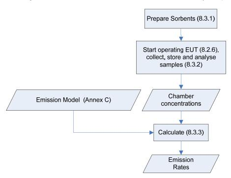
Figure 2 — Determination method for VOC, carbonyl compounds
