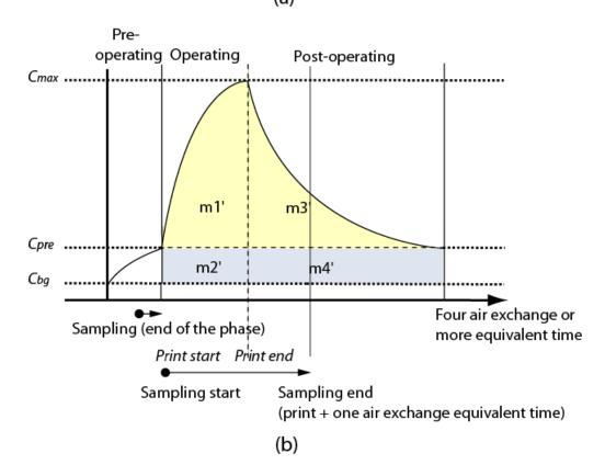
Figure C.2 — Model for equilibrium and constant  $C_{\rm o}$  (a) and (b) RAL-UZ 122 Option model
