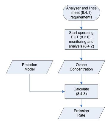
Figure 3 — Determination method for ozone
