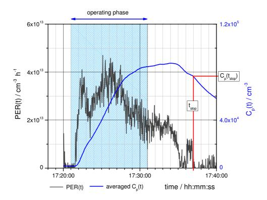
Figure 7 — Diagram of PER(t) and C<sub>p</sub>(t)
