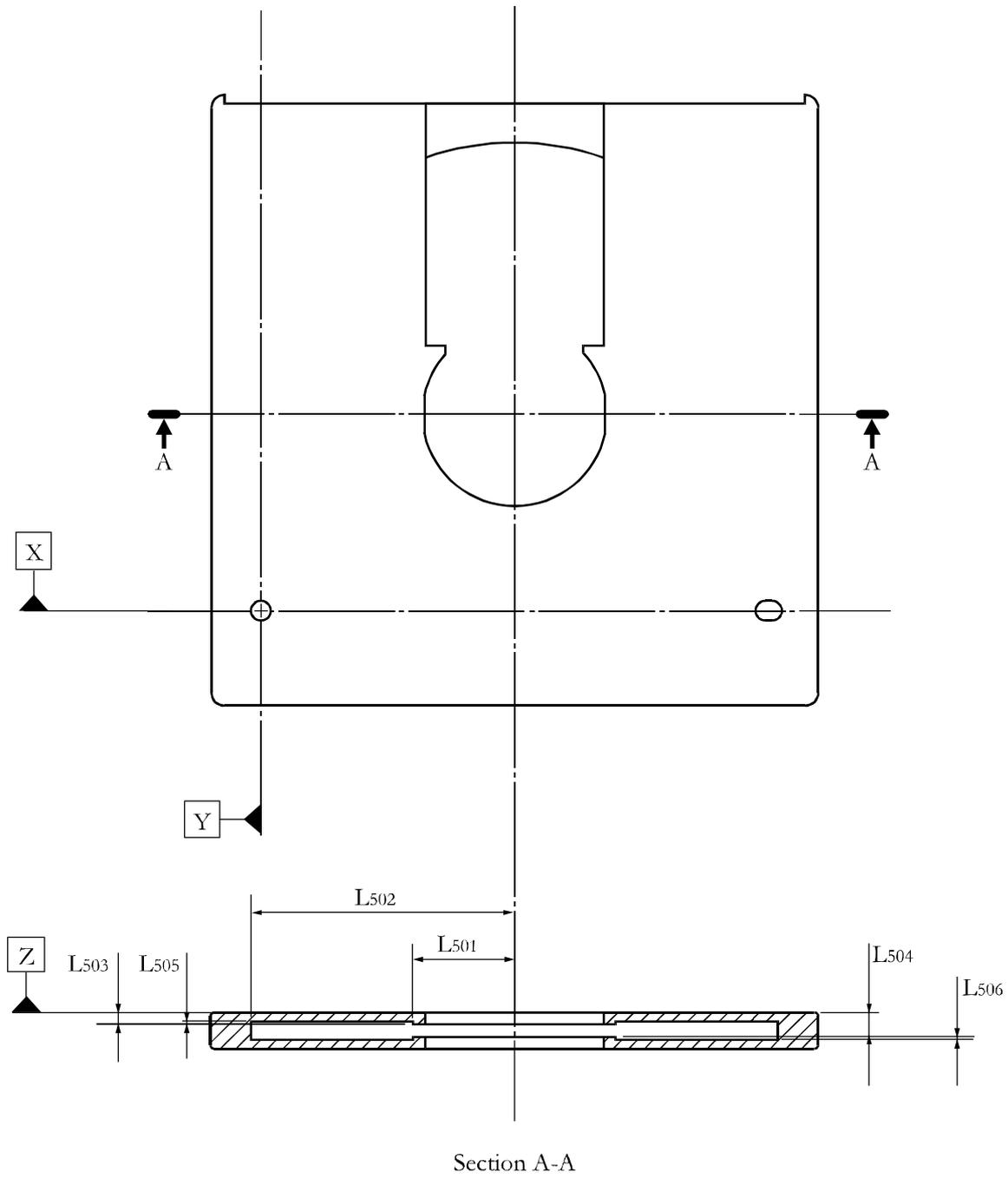
**Figure 51 - Inner dimensions of the case**
