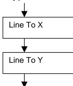
The Glyph Line To command draws a line to the specified point.
