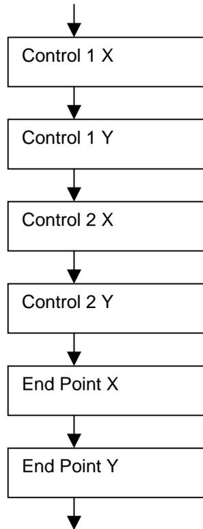
The Glyph Curve To command draws a curve to the specified point. The control points are used to determine the curve.
