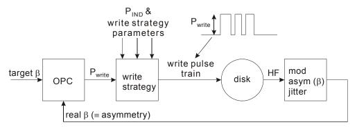
Figure I.1 - Schematical diagram of OPC procedure
