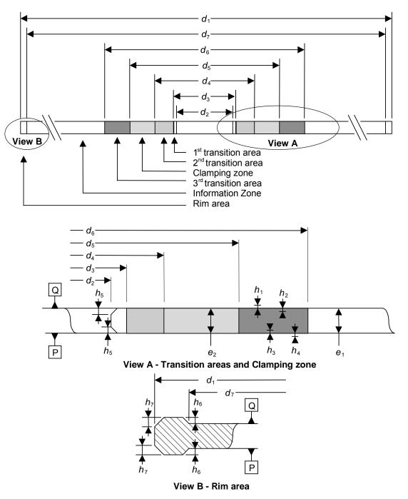
Figure 6 - Physical disk dimensions
