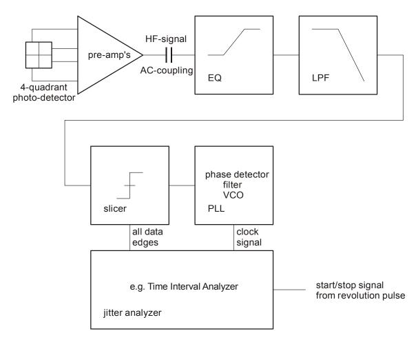
Figure E.1 - General diagram for jitter measurement
