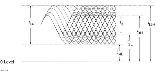
Figure 43 - Signals from spaces and marks in Read channel 1
