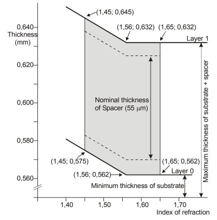
Figure 9 - Thickness of the substrate
