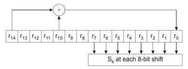
Figure 13 - Feedback shift register
