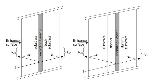
Figure K.2 - Example of samples for measuring absorption and transmission
