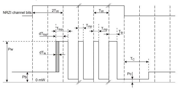
Figure G.1 - Write pulse waveform
