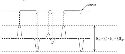
Figure 46 - Tangential push-pull signal
