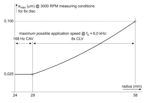
Figure L.5 - Illustration of 8x disk radial residual tracking errors and application speed
