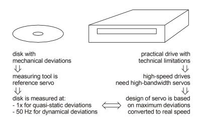
Figure L.1 - Illustration of disk measurement and drive design
