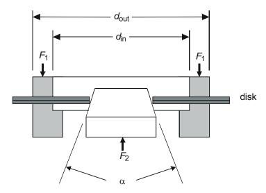
Figure 3 - Clamping and chucking conditions
