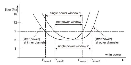
Figure 42 - Example of the write power windows
