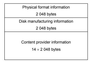
Figure 31 - Structure of a Control Data Block
