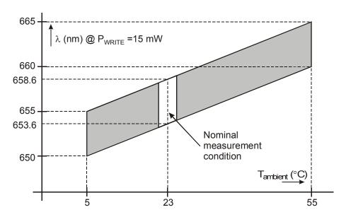
Figure K.1 - Wavelength/Temperature diagram indicating the disk operating conditions
