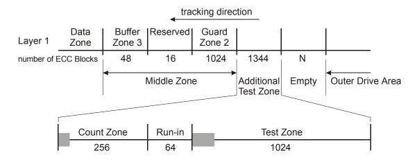
Figure 25 - Additional Testing Zone on Layer 1
