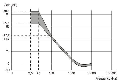
Figure 4 - Reference servo for axial tracking
