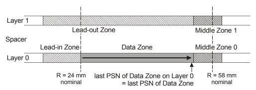
Figure 38 - Example of Finalized disk with only data on Layer 0
