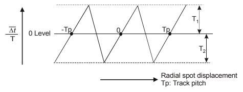
Figure 45 - Differential phase tracking error signal
