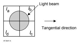
Figure 44 - Quadrant photo detector
