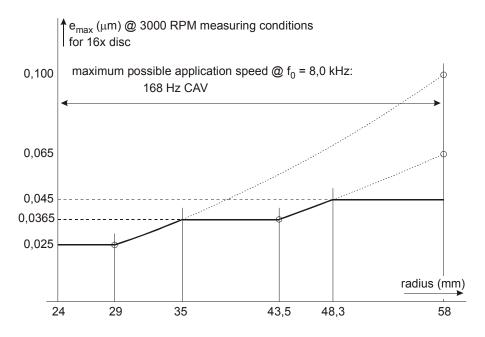
Figure L.7 - Illustration of 16x disk radial residual tracking errors and application speed
