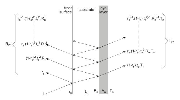
Figure K.3 - Definitions of reflectivity, transmission and absorption
