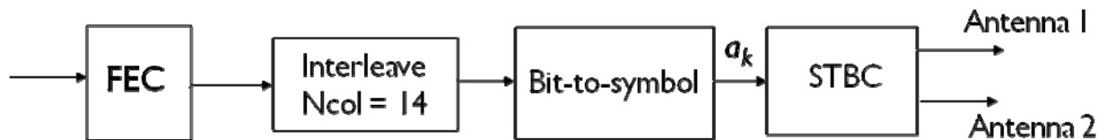
Figure 46 — Block diagram of Space Time Block Code (STBC) transmission scheme
