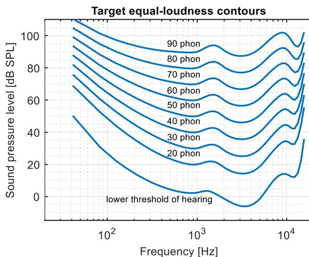
Figure F.2 — Equal loudness contours (ISO 226:2003) used as target for the filter transfer function
