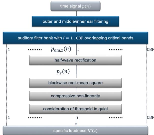
Figure F.1 — Basic hearing model structure
