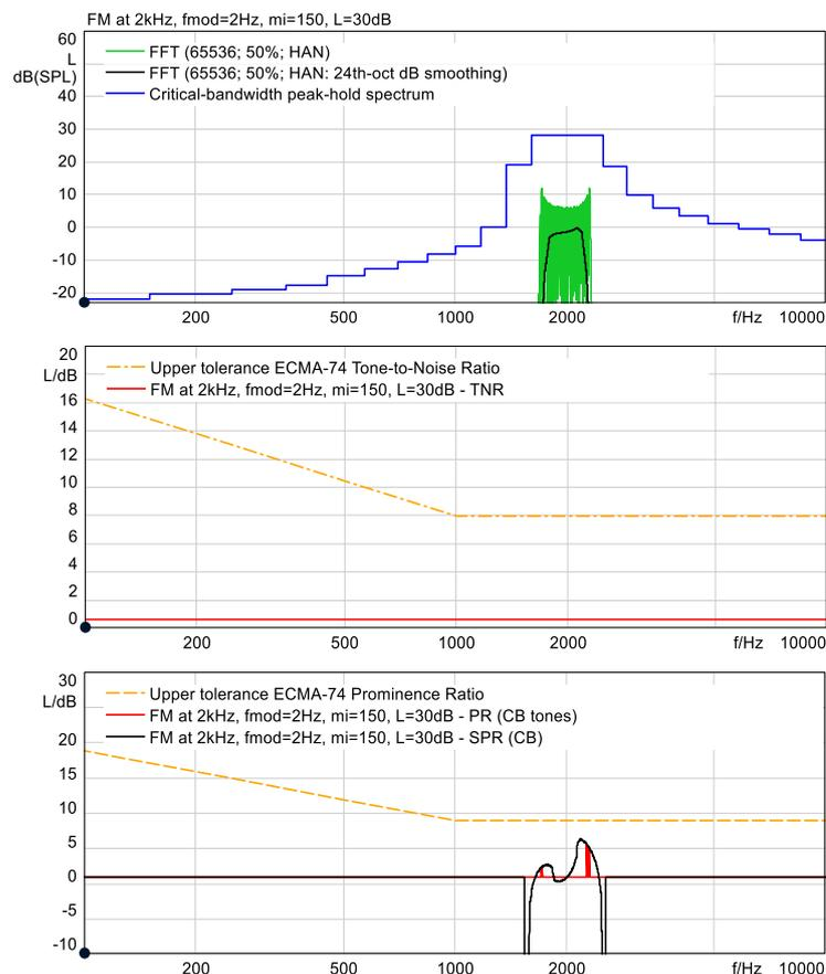
**Figure G.3 — Top: Different spectral representations (FFT and smoothed FFT) of a frequency-modulated tone; Middle: corresponding TNR results (scale gives dB of tonal audibility); Bottom: corresponding PR values tones-only (according to Annex D) using critical bands (CB) and complete SPR not constrained only to pure tones results**
