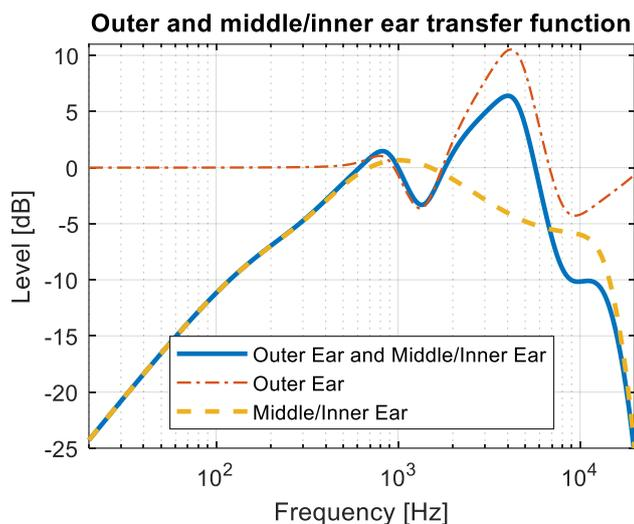
**Figure F.3 — Transfer function of the outer and middle/inner ear filter**
