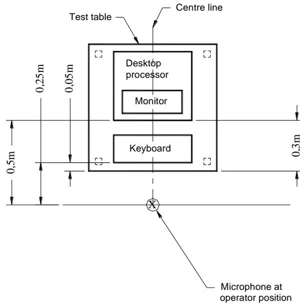
Figure C.4a — Installation for system comprising "flat" table-top equipment
