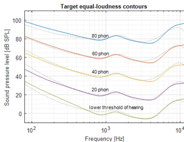
**Figure F.5 — Results for the equal-loudness contours. The dotted lines show the target equal-loudness contours, the solid lines are the equal-loudness contours obtained with the hearing model**
