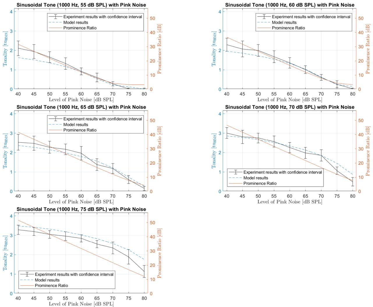
**Figure G.5 — Psychoacoustic tonality and Prominence Ratio compared to results of listening tests**
