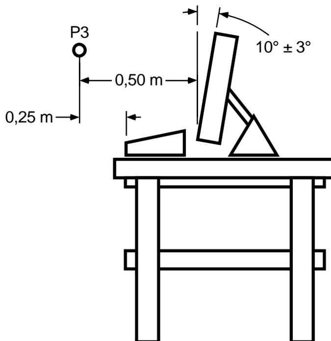
Figure C.4d — Screen angle for all-in-one system
