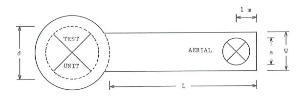
D = d + 2 m, where d = maximum test unit dimension W = a + 1 m, where a = maximum aerial dimension L = 3 m or 20 m or 30 m
