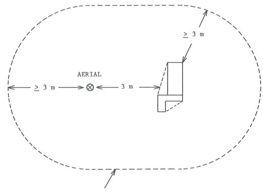
Surrounding boundary. Volume above earth to be free of reflecting objects  $\geq 3$  m above the test sample or aerial, whichever is greater.
