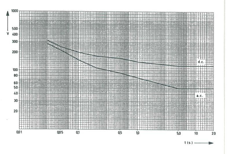
Figure 41B - Maximum prospective touch voltage duration curves according to table 41A
