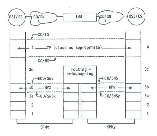
Figure 1 - Layered Structure for Connection Oriented/Connection Oriented Interworking within the OSI Network Layer to achieve a Connection Oriented Network Service (OSC1).
