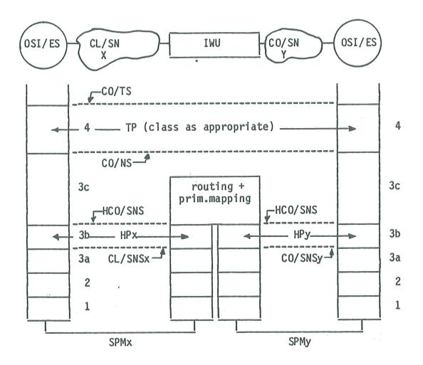
Figure 3 - Layered Structure for Connectionless/Connection Oriented Interworking within the OSI Network Layer to achieve a Connection Oriented Network Service (OSC3).
