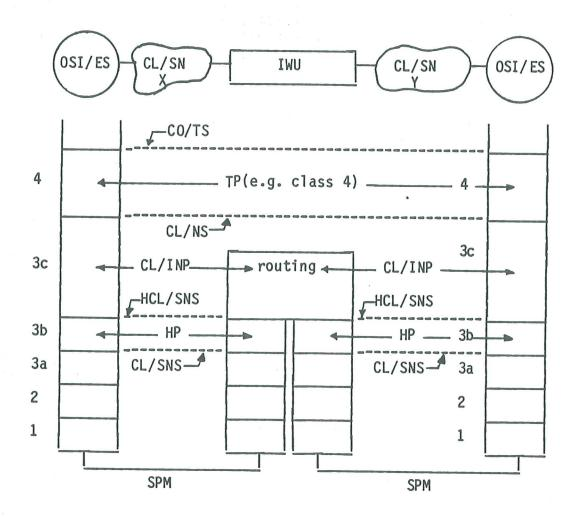
Figure 2 - Layered Structure for Connectionless/Connectionless Interworking within the OSI Network Layer to achieve a Connectionless Network Service (OSC2).
