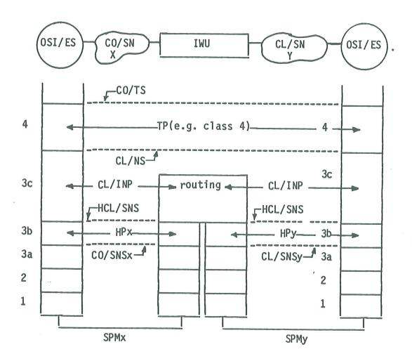
Figure 5 - Layered Structure for Connection Oriented/Connectionless Interworking within the OSI Network Layer to achieve a Connectionless Network Service (OSC4).
