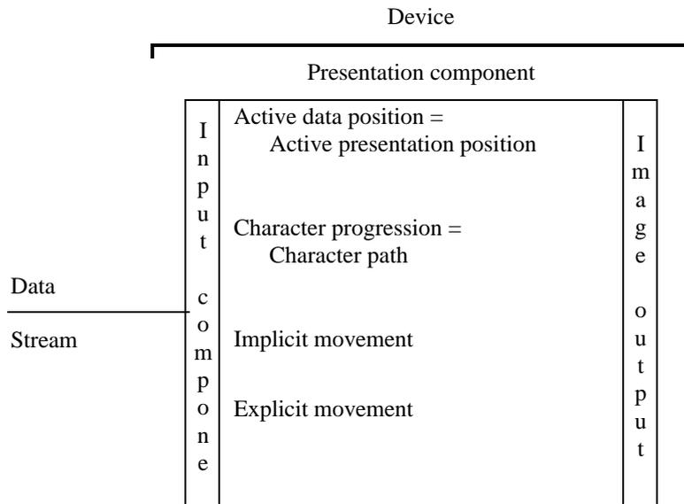
Figure 3 - Bi-directional device with presentation component only
