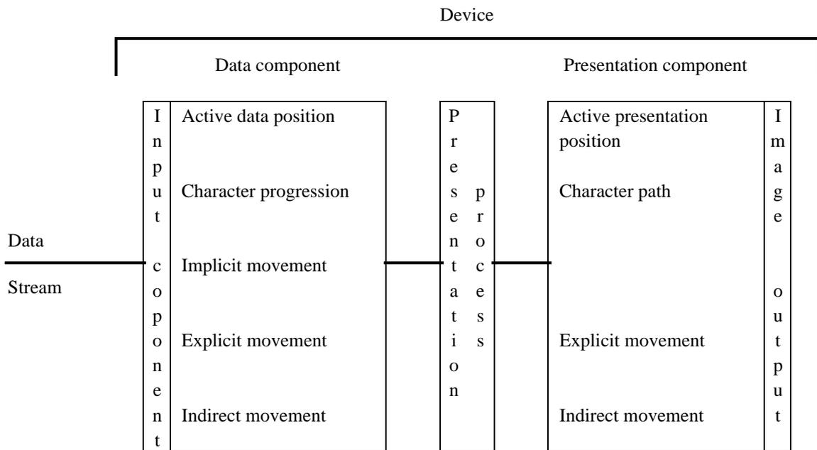
Figure 2 - Bi-directional device with data and presentation component
