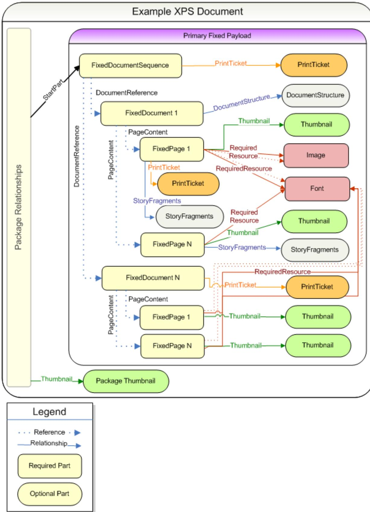
Figure 2: Internal OpenXPS Document structure builds on the Open Packaging Conventions Standard
