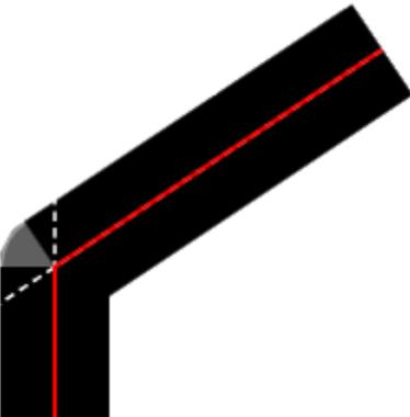
Figure 18–24. Mitered line join with right angle and miter limit of 2.0
